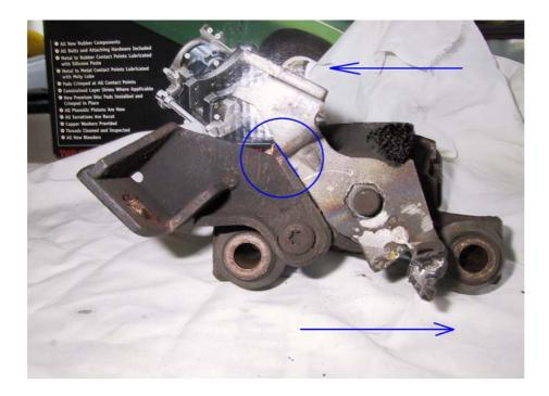
But when the lever is operated in a clockwise direction, we have a fair amount of travel before the lever catches on the lower section of the handbrake bracket.
