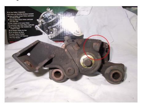
The purpose of this missing casting is to limit the clockwise/counter-clockwise movement of the handbrake actuator arm.
