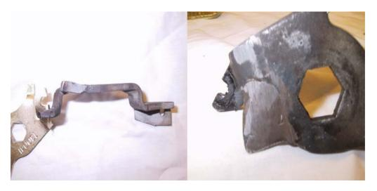
This is what they look like fitted. If you look close enough, you'll be able to see the mod to the lever i.e the picture on the left has no gap between the lever and the bracket (hand brake off). Right shows a gap between the lever and the bracket (hand brake on).
