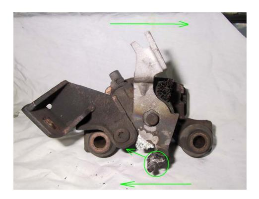
So our solution to this problem, was to weld a triangle section of steel onto the lower section of the actuator arm, which when operated in a clockwise direction, catches against the lower section of the handbrake bracket. See below.
